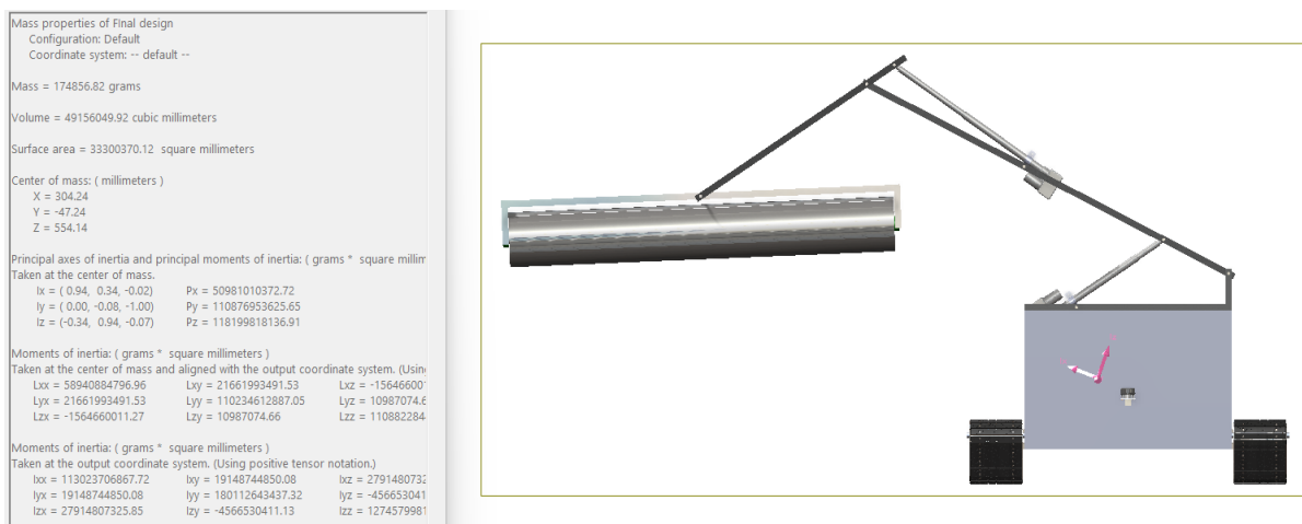
Figure 3.6.1: the right view of the robot and the center of mass is nearly at the center of the robot
