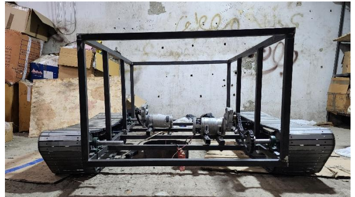
Figure 2.6.25: Final shape after assembling the two chains
