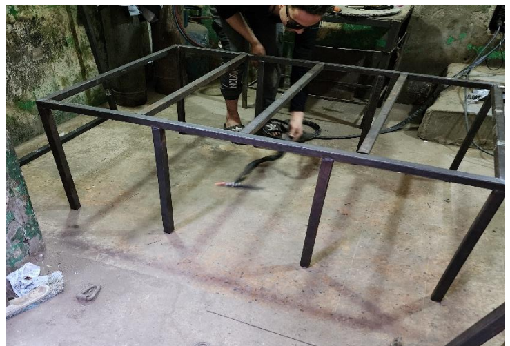
Figure 2.6.3: Chassis during welding process
