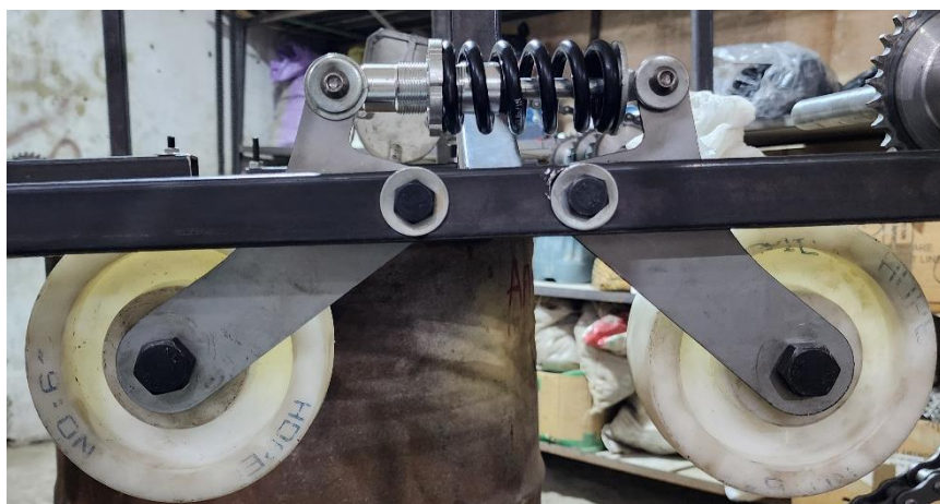
Figure 2.6.15: Suspension mechanism testing phase
