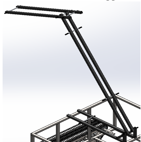
Figure 3.1.5: shows the arm of the robot constructed of two links and a base
