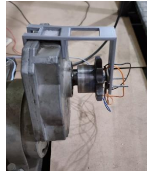
Figure 2.6.13: Encoder holder mounted on the motor
