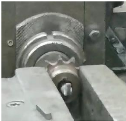
Figure 2.6.11: Sprocket's key opening process
