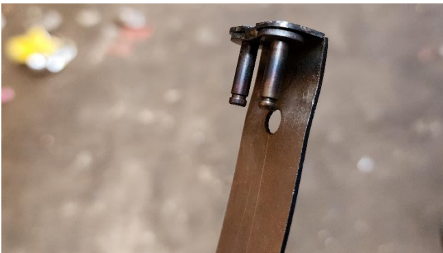
Figure 2.6.21: Welding test of the sheet metal to the chain
