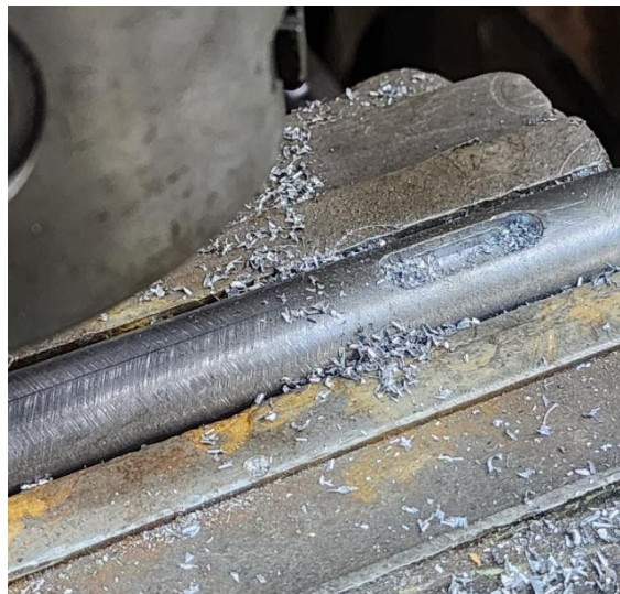
Figure 2.6.8: Keys slot opening process
