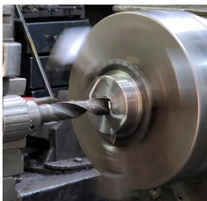
Figure 2.6.10: Sprocket's turning process
