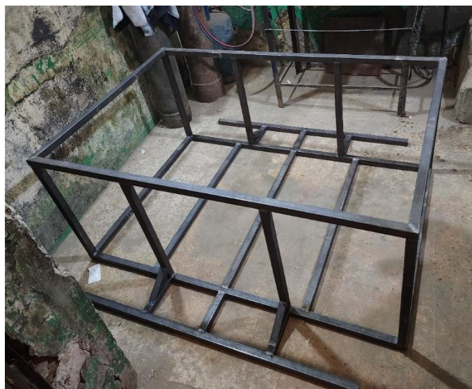
Figure 2.6.4: Final welded chassis
