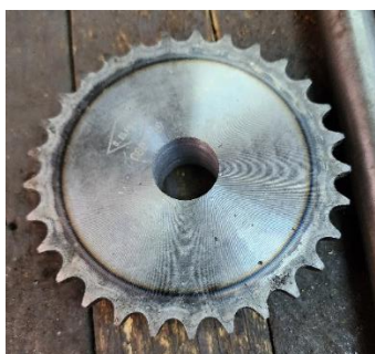
Figure 2.6.9: Sprocket before machining
