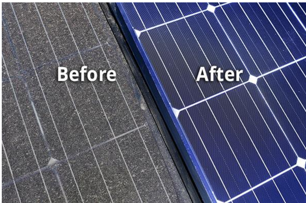
Figure 1.3.1: Close-up image of dirty vs. clean solar panels
