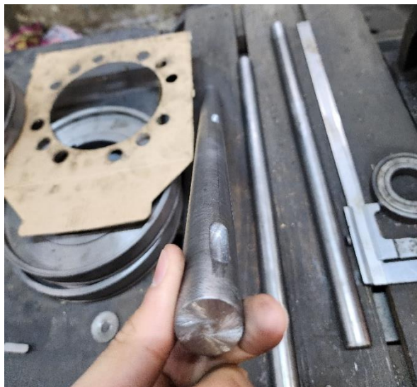
Figure 2.6.7: Shafts after opening keys slots
