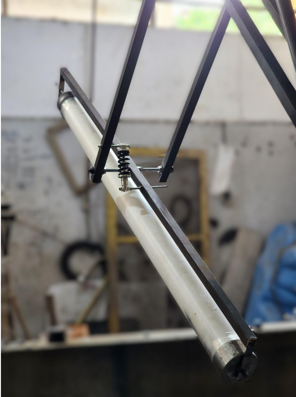
Figure 3.1.7: shows the design of the brush and the brush holder with the suspension in reality
