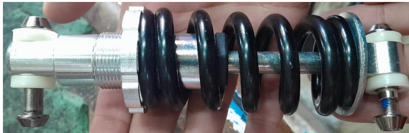
Figure 2.6.16: Suspension Spring module
