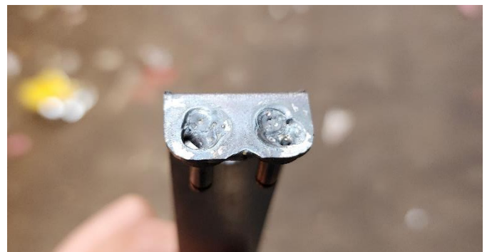
Figure 2.6.22: Welding test of the sheet metal to the chain
